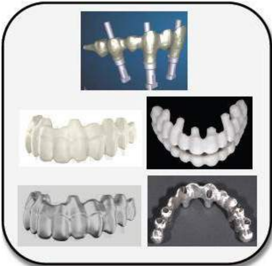
Figure 15. CAD CAM fabricated frameworks for fixed prosthesis. Top: virtual design, Middle: Zirconia framework with or without buccal flange material, Bottom: Titanium framework with or without buccal flange material
