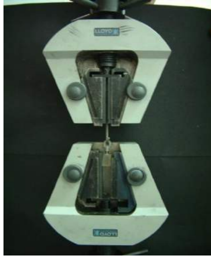
Figure 10. An example for a pull-out test setup. In this experiment the maximum pull-out force of a luting agent is tested. Note the hookup system to apply axial force.
