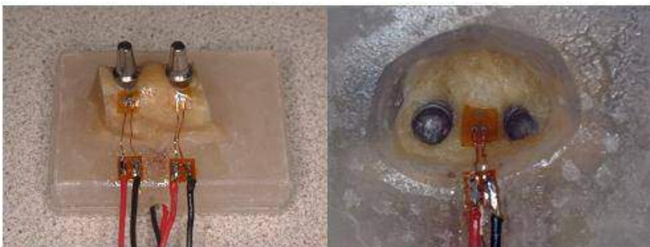
Figure 15. Strain-gauge analyses in a simulation of advanced surgical approach applied in maxillary posterior region (a and b).
