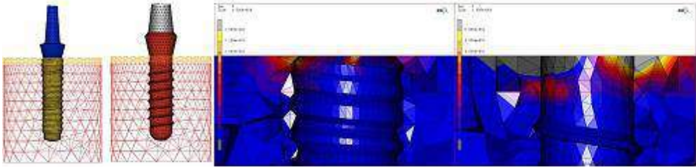
Figure 7. Quantitative and qualitative comparison of load transfer of bone- and soft tissue-level implants in a mathematical simulation (a to c).
