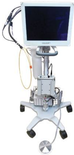
Figure 2.1 The glass fiber endoscope for use in nonsurgical minimally invasive periodontal therapy is shown. Source: Courtesy of Dr. John Kwan.
