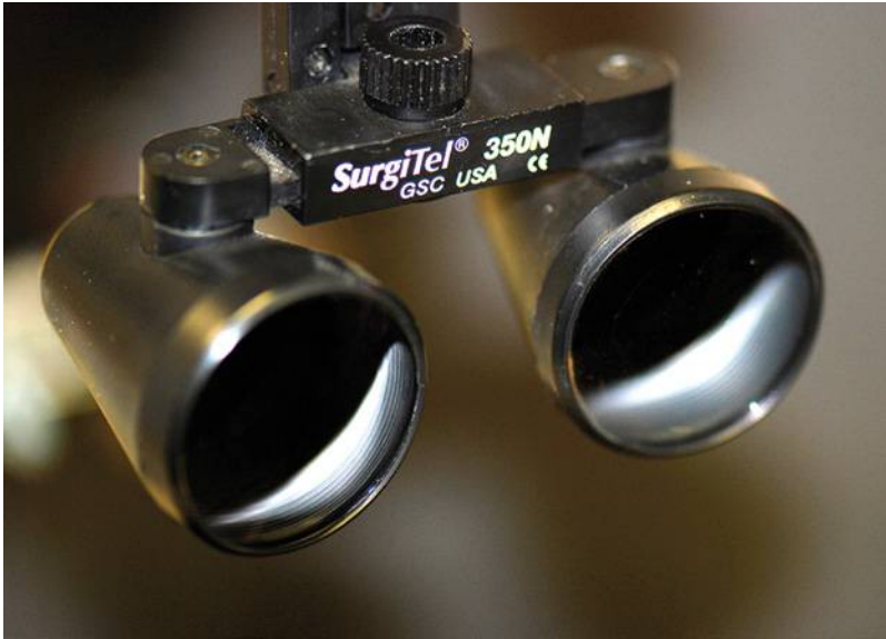
Figure 2.3 A surgical telescope or loupe with an integral light is shown. Source: Courtesy of Dr. Jonathan Blansett.
