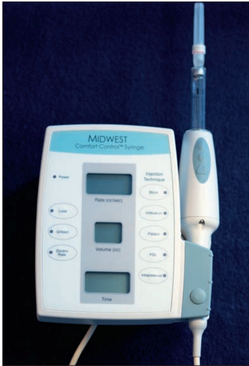
Fig 4-14 The Comfort Control Syringe is an electronic delivery system for local anesthesia and has five different injection rates that are preprogrammed into the system.
